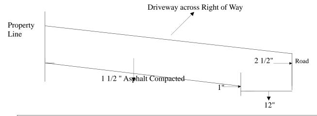
Note: A clean cut must be made on the existing street, with no dirt between the street and driveway connection. Connection must be flush with existing asphalt.
